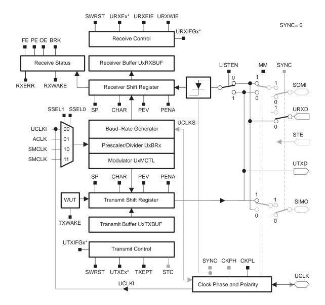
Figure 13-1. USART Block Diagram: UART Mode
